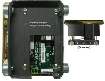
FIG. 5 Rear and side view of magnetic housing
